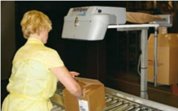
A modified Shooter machine on a swivel puts the packaging material closer to the packer.
